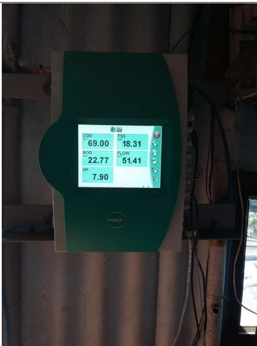
Online monitoring system for sugar ETP effluent sample
