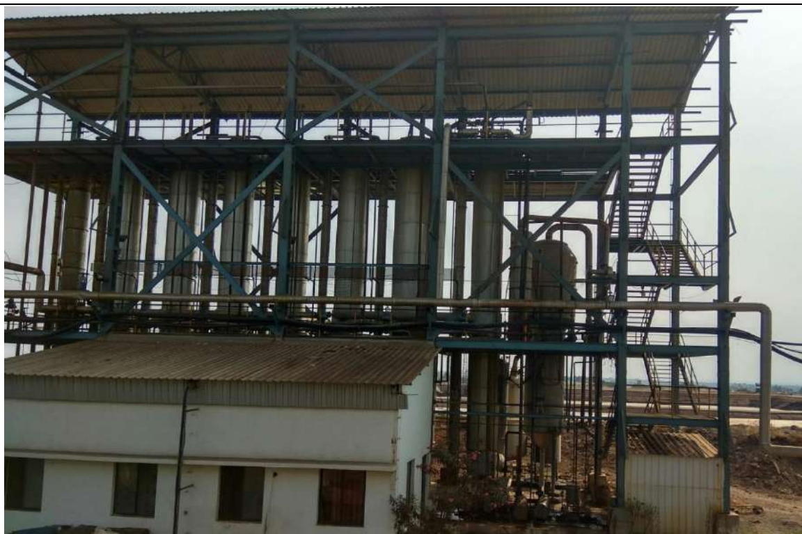
Multi Effect Falling Film Evaporation Plant (Capacity 900kld)
